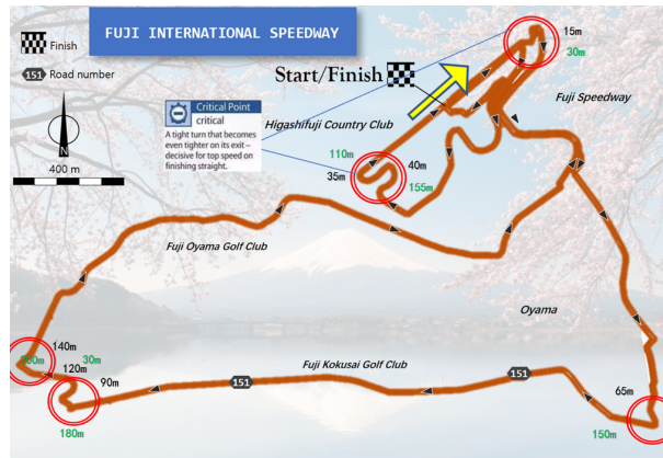
Figure 11: Fuji international speedway. The seven sharp turns are marked with red circles. The black numbers next to the corners represent the radius of curvature, and the green numbers represent the length of the corner.
